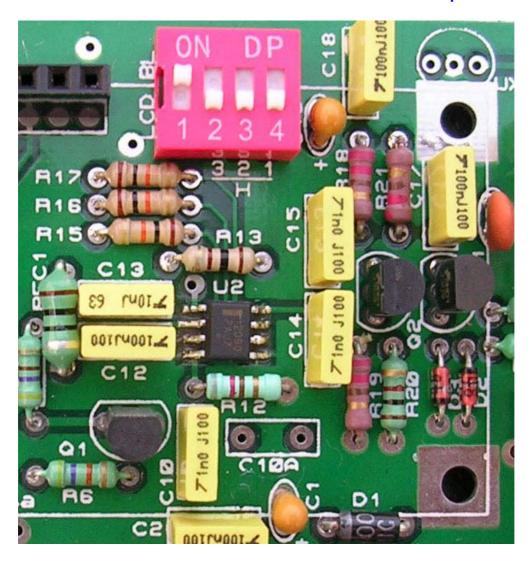
400MHZ completed frequency counter is visible in above picture. If you wish to use FC2A to 40mhz only, it is achieved by not installing C10 and installing same capacitor at C10A.
